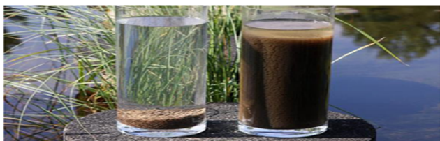
Figure 2: Comparison of sedimentation between Nereda and conventional, respectively.
