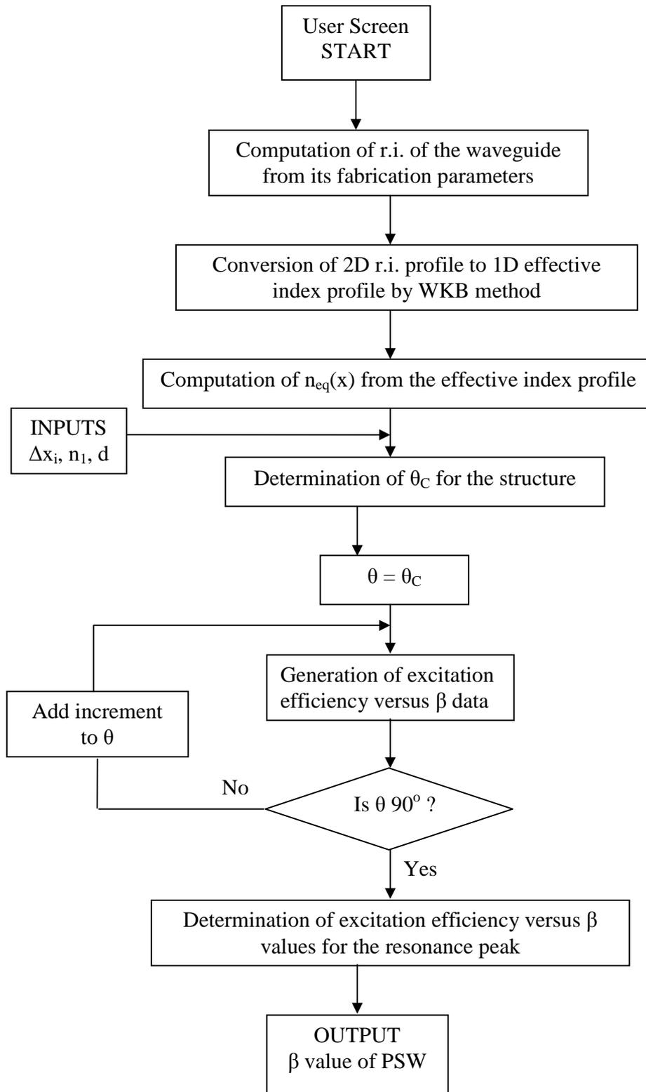
Figure 2 Flow-chart for computation of the propagation constant of Ti:LiNbO<sub>3</sub> PSW.
