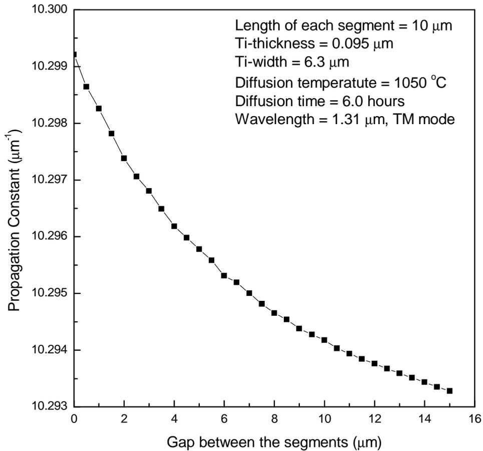
Figure 3 Computed propagation constant versus gap between the segments of a Ti:LiNbO<sub>3</sub> PSW.
