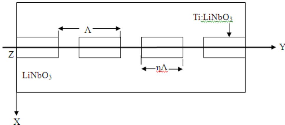
Figure 1 Periodically segmented waveguide (PSW).
