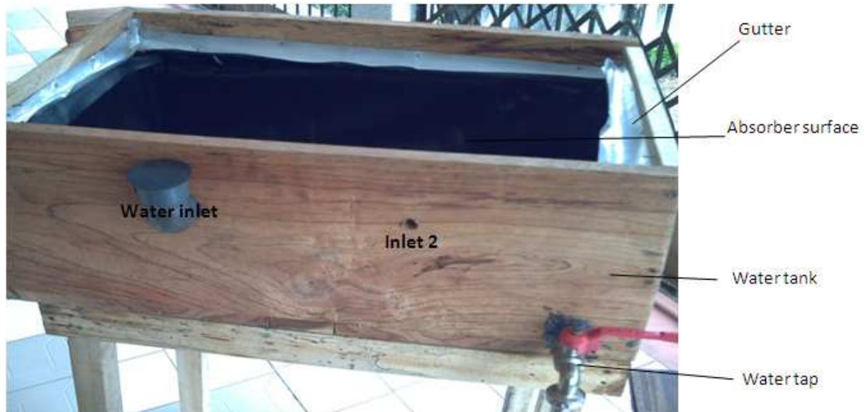
Figure 1. The rectangular water tank on top of RSWD stand
