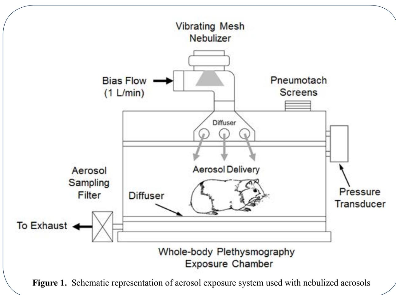
**Figure 1.** Schematic representation of aerosol exposure system used with nebulized aerosols
